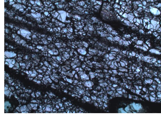
Sample U831-09 from the Udachnaya kimberlite structure. Top left is an image of the thin section clearly showing a mylonitic pattern with olivine sheared into striations. Above is the sample zoomed in on a petrographic microscope showing individual olivine grains and banding. On the left is an image from the SEM of individual olivine grains with a scale of 300 micrometers.
